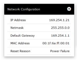
To change the network configuration, click on the gear icon in the upper right hand portion of the screen. A dialog box will pop up, asking you for the updated IP address. After you click 'Accept Changes', the IP address will be saved and will take effect immediately.
