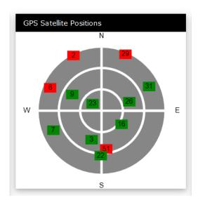
**GPS Satellite Positions:** This section of the screen is useful to determine if you are having visibility problems with a portion of the sky.
