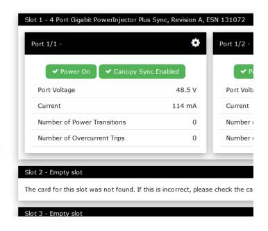
If a slot is empty (doesn't contain a board), then the web interface will display this fact.
