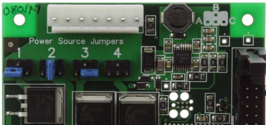
To select a particular power source, set the jumper as appropriate for the power source you are selecting for that port. The left position selects Power source A, the center position selects power source B, and the right position selects power source C. With no jumper in place the port will not be powered.
