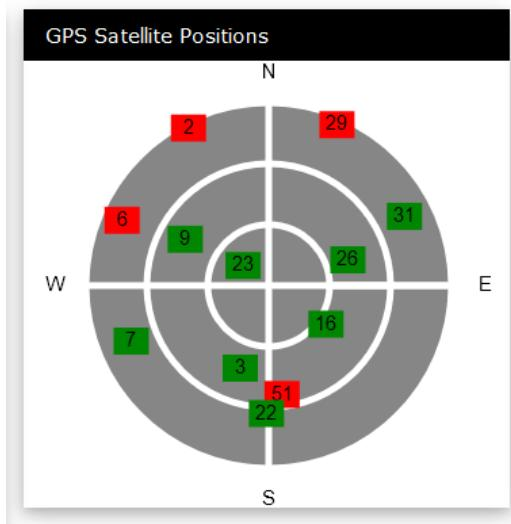
**GPS Satellite Positions:** This section of the screen is used to determine if you are having visibility problems with a portion of the sky.
